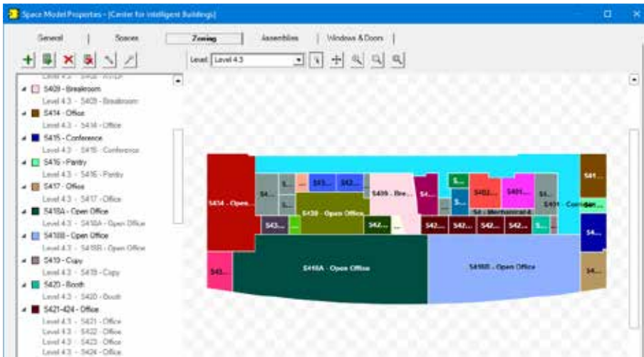
The HAP v6 offers visual, point-and-click features for rapidly grouping rooms into HVAC control zones, Carrier said
